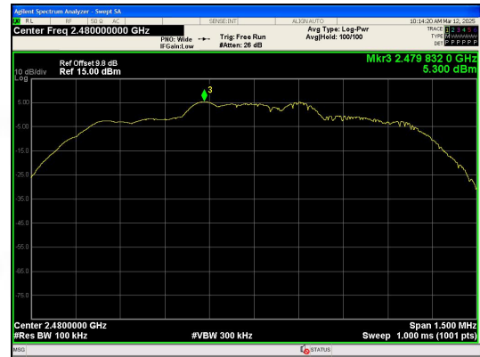
In-Band Reference Level \pi/4 DQPSK_2-DH1_Channel 78
