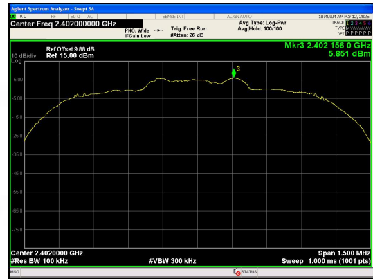
In-Band Reference Level \pi/4 DQPSK_2-DH5_Channel 0
