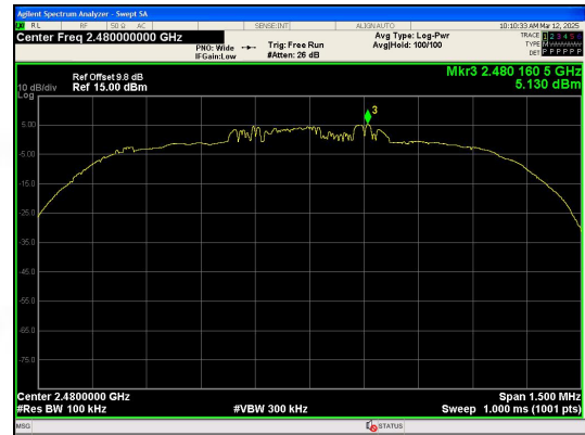
In-Band Reference Level \pi/4 DQPSK_2-DH5_Channel 78
