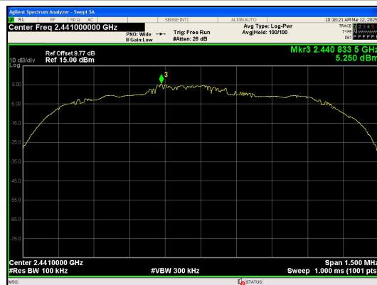
In-Band Reference Level 8DPSK_3-DH3_Channel 39
