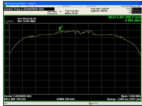
In-Band Reference Level 8DPSK_3-DH3_Channel 0
