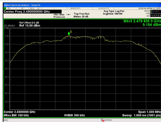
In-Band Reference Level 8DPSK_3-DH3_Channel 78
