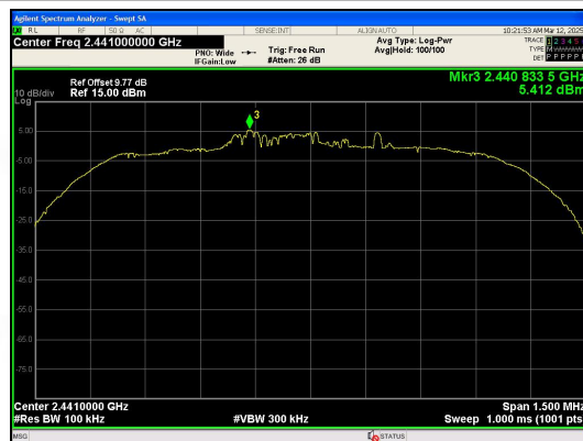
In-Band Reference Level \pi/4 DQPSK_2-DH5_Channel 39
