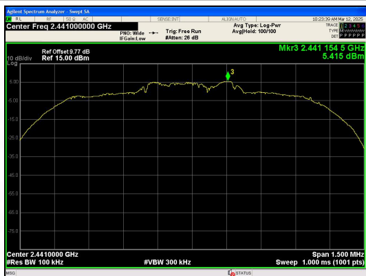
In-Band Reference Level \pi/4 DQPSK_2-DH3_Channel 39
