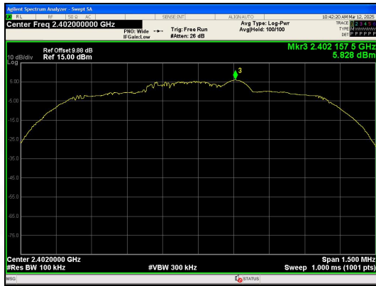
In-Band Reference Level \pi/4 DQPSK_2-DH3_Channel 0
