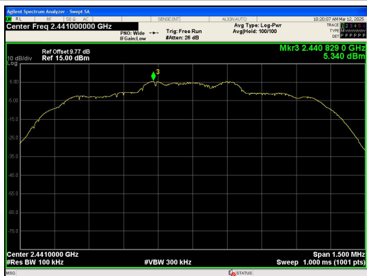
In-Band Reference Level 8DPSK_3-DH1_Channel 39
