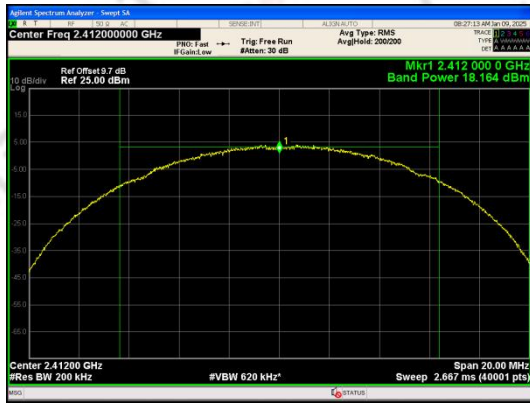
Conducted AVG output power IEEE 802.11b_Channel 1_Antenna 0
