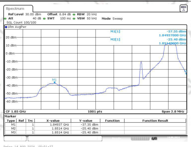
Band2 QPSK BW=1.4MHz Channel=18607 RB Size=1 Position=#Max NVNT
