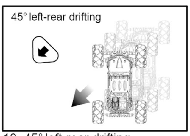
10. 45° left-rear drifting Press the 45° Left-Rear Drifting button to make the vehicle drift to the left-rear at an angle of 45 degrees. Press and hold this button will make the vehicle keep drifting to the left-rear at an angle of 45 degrees.
