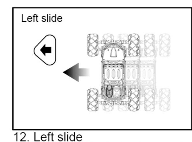
Press the Left Slide button to make the vehicle slide to the left. Press and hold this button will make the vehicle keep sliding to the left.
