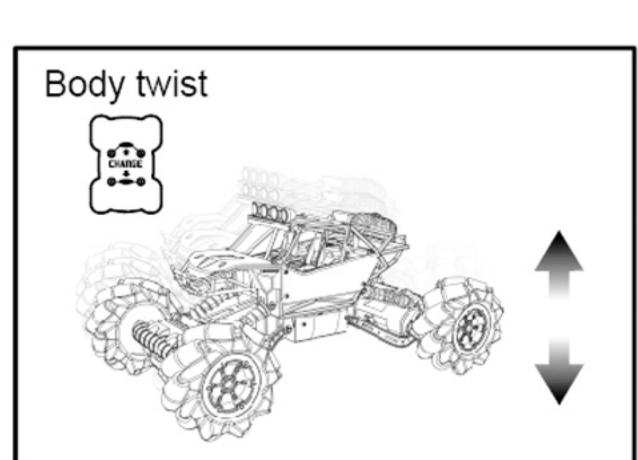
3. Body twist Press the Change button once to lower the vehicle body. Press the Change button again will make the vehicle return
