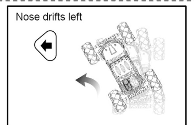
Nose drifts left Press the Nose Drifts Left button to make the vehicle's nose drift to the left. Press and hold this button will make the nose keep drifting left.
