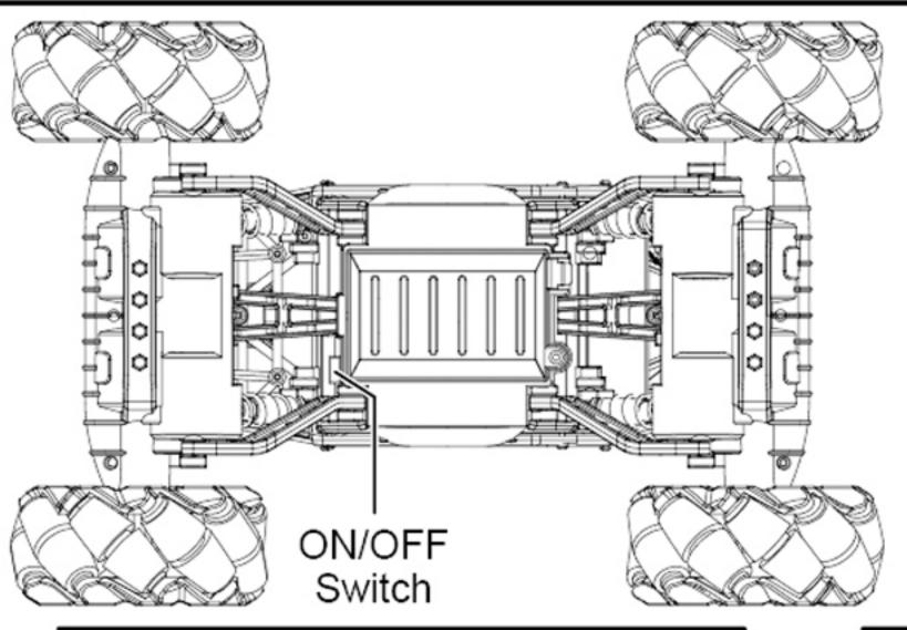
Power ON: Turn on the vehicle and then the transmitter. The light on transmitter will turn off to indicate the transmitter and the vehicle is linked. Remote control distance: more than 20 meters. Operating time: approx. 20-30 minutes with fully charged battery.
