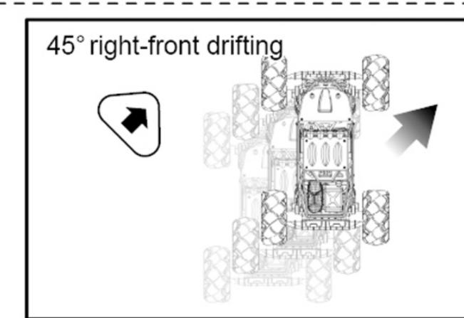
9. 45° right-front drifting Press the 45° Right-Front Drifting button to make the vehicle drift to the right-front at an angle of 45 degrees. Press and hold this button will make the vehicle keep drifting to the right-front at an angle of 45 degrees.
