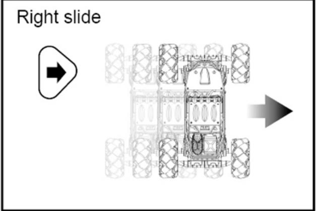
13. Right slide Press the Right Slide button to make the vehicle slide to the right. Press and hold this button will make the vehicle keep sliding to the right.
