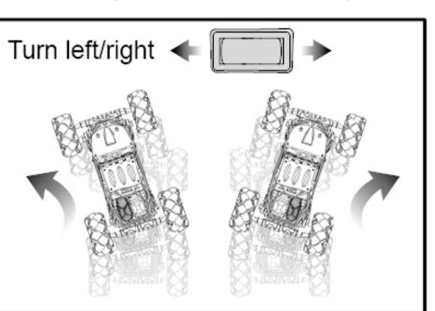
Push the left stick to the left to turn left and to the right to turn right. Push and make the vehicle keep turning left/right.
