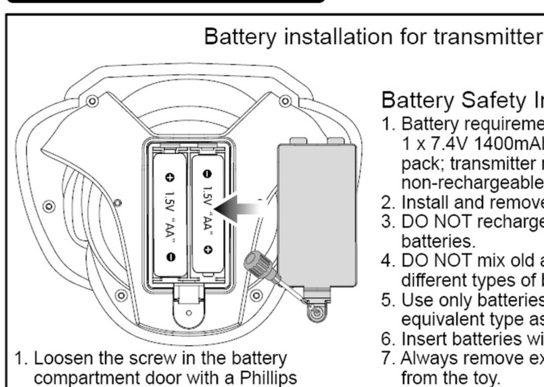
2. Install 2 x 1.5 V "AA" batteries with
