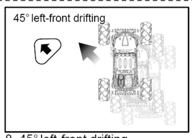
8. 45° left-front drifting Press the 45° Left-Front Drifting button to make the vehicle drift to the left-front at an angle of 45 degrees. Press and hold this button will make the vehicle keep drifting to the left-front at an angle of 45 degrees.
