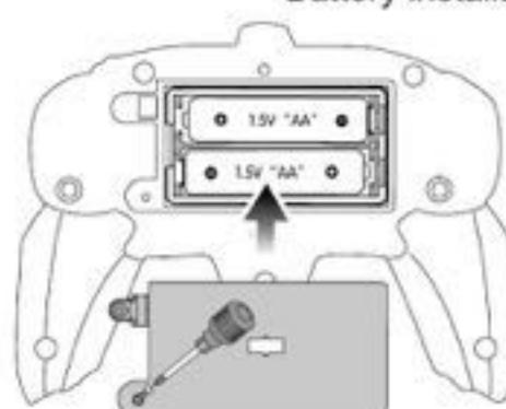
1. Loosen the screw in the battery compartment door with a Phillips screwdriver.
