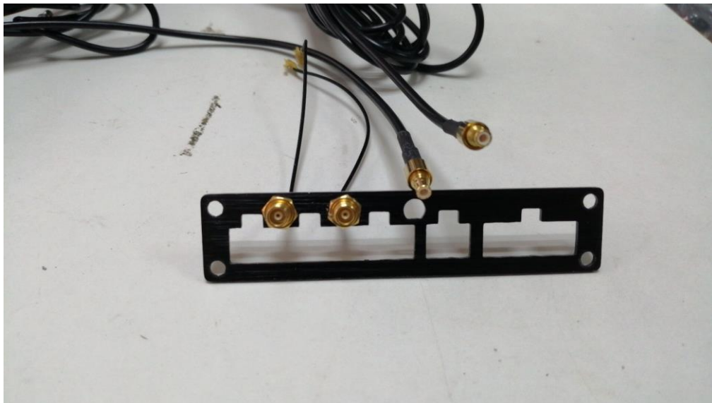
Extenal Antenna Connector: MCX Connector
