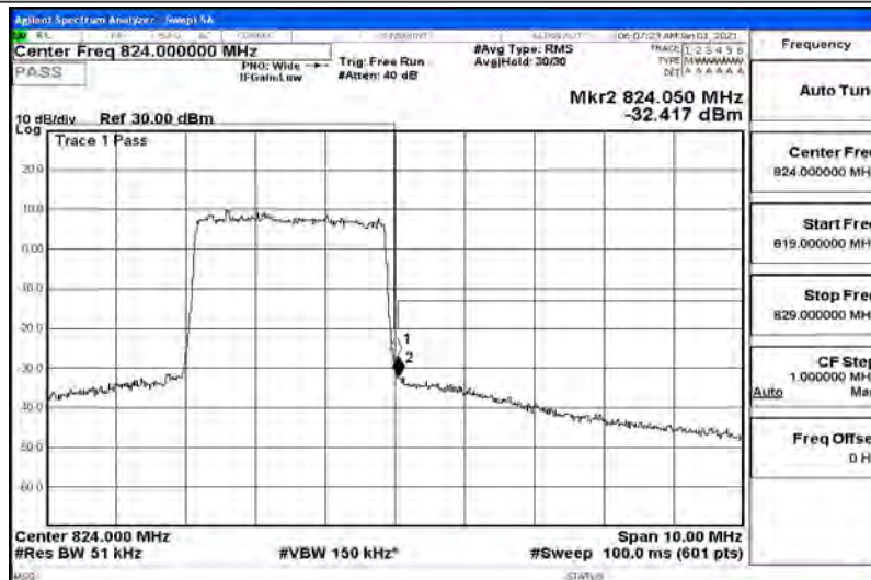
Band Edge Test Graph(s) (Channel Bandwidth: 3 MHz)_HCH_16QAM
