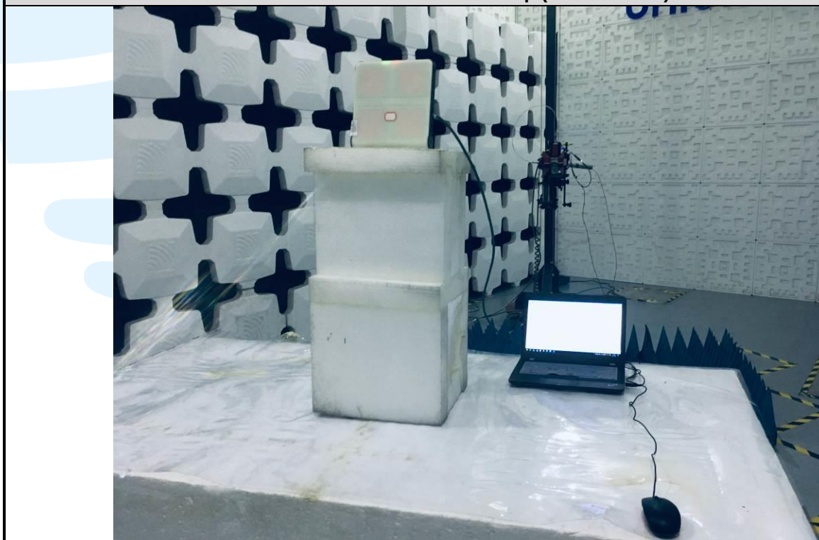
Radiated emission Test Setup (Above 1 GHz)
