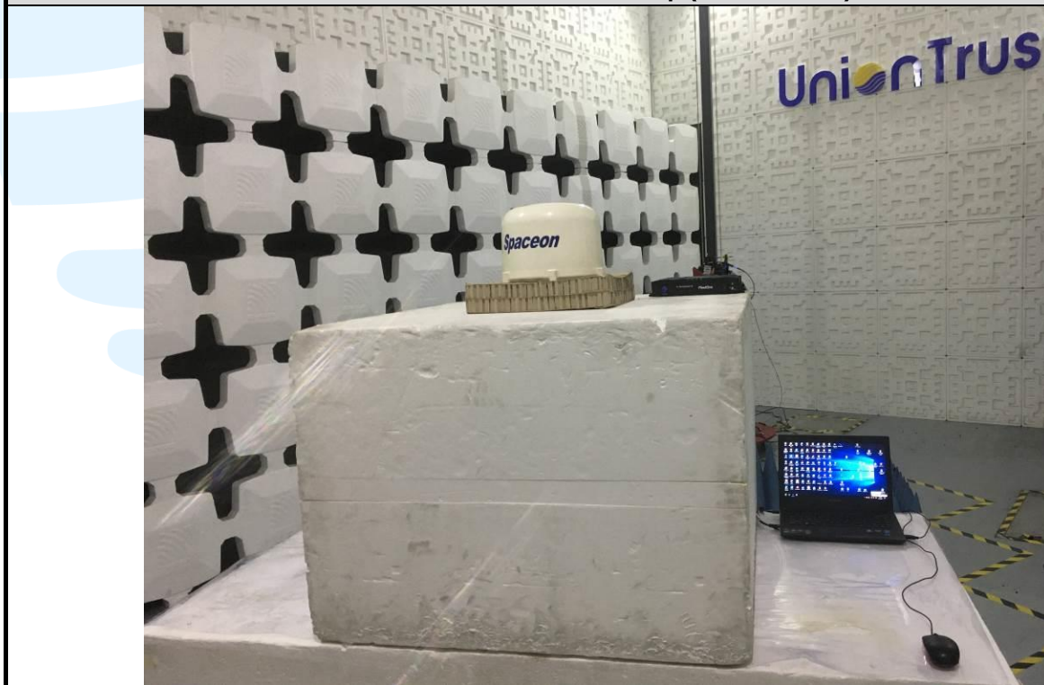
Radiated emission Test Setup (Above 1 GHz)
