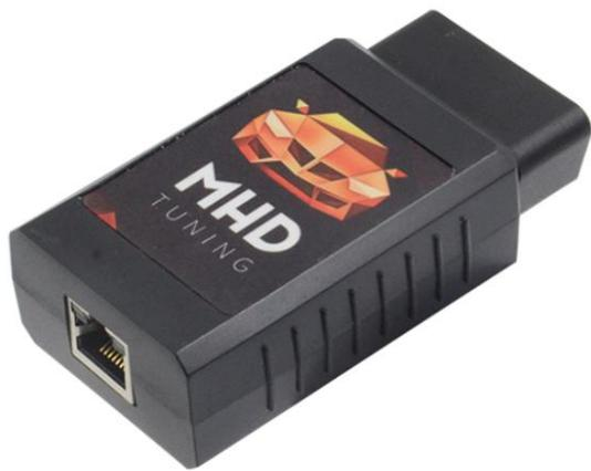
MHD OBD2 Wifi Flasher was specially developed and designed to operate the Ethernet OBD2 diagnostic and coding features via wired J2534 port and wireless via an embedded module based on the universal serial interface network standard,built-in TCP / IP protocol stack, enabling the user serial port, Ethernet, wireless network (wifi) interface between the conversions. the traditional serial devices do not demand to change any configuration, data can be transmitted through the
