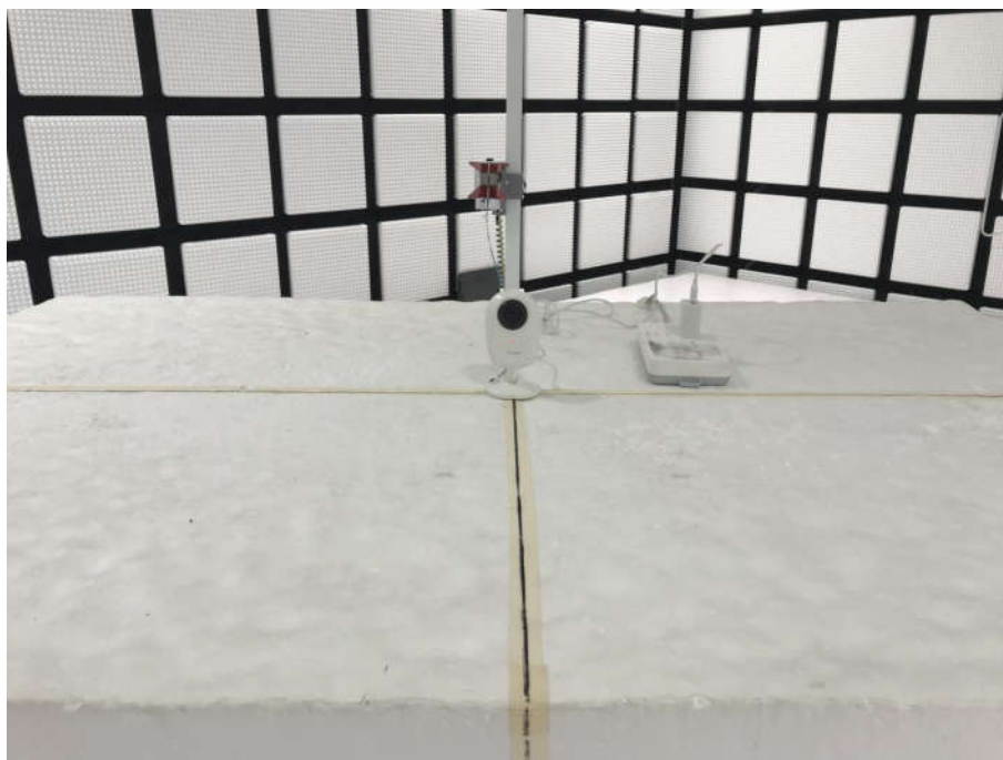
Radiated spurious emission Test Setup-2(Above 1GHz)
