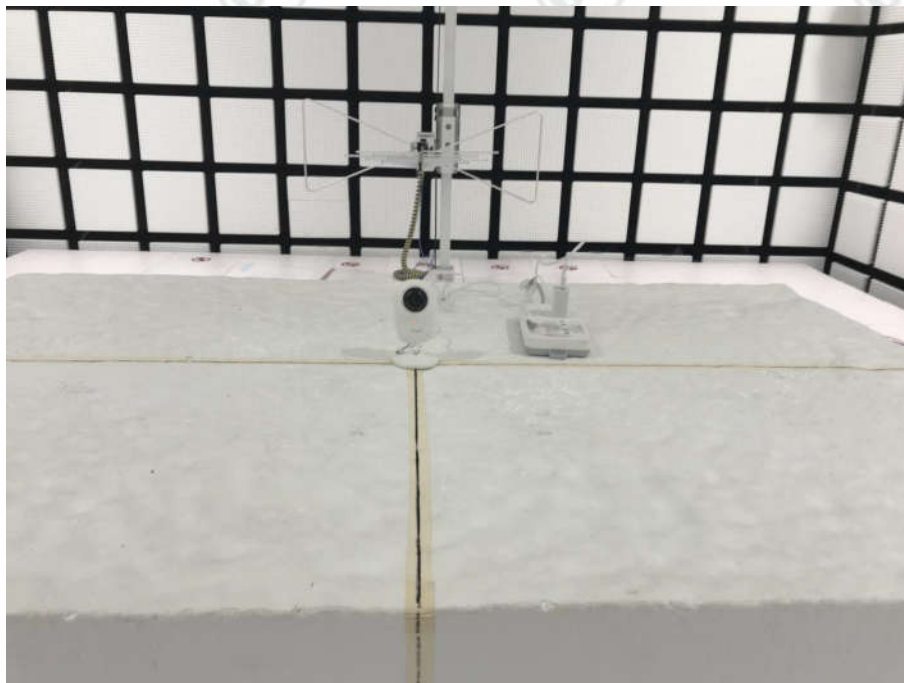
Radiated spurious emission Test Setup-1(Below 1GHz)
