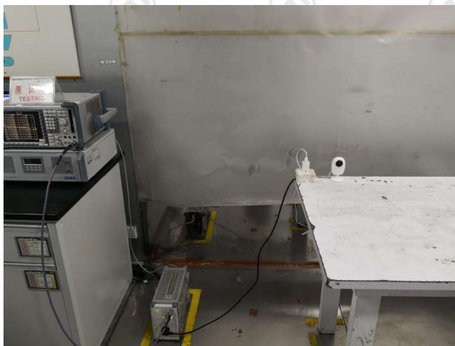
Conducted Emissions Test Setup
