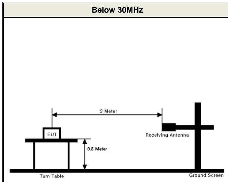
**- Procedure:** The radiated emission was tested according to the **section 6.4 of the ANSI C63.10-2013**.
