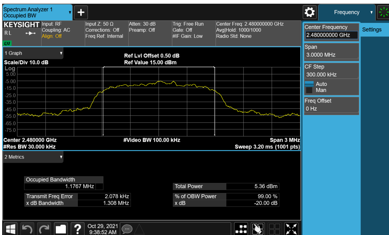
Figure 15: 20dB Bandwidth and 99% Bandwidth, 2480MHz, 8-DPSK
