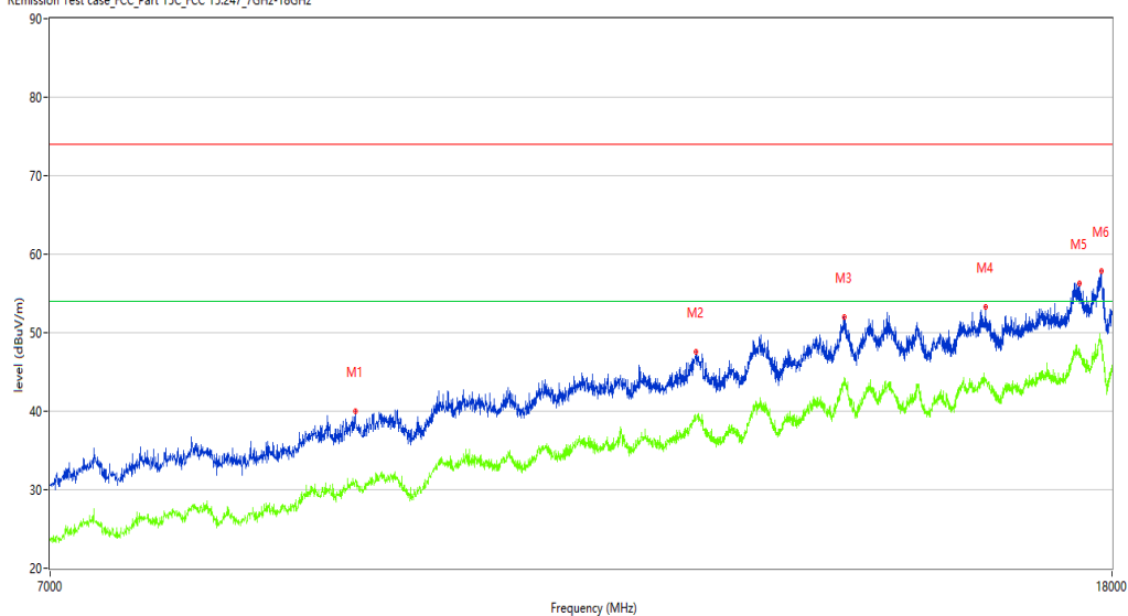
R Emission Test case_FCC_Part 15C_FCC 15.247_7GHz-18GHz
