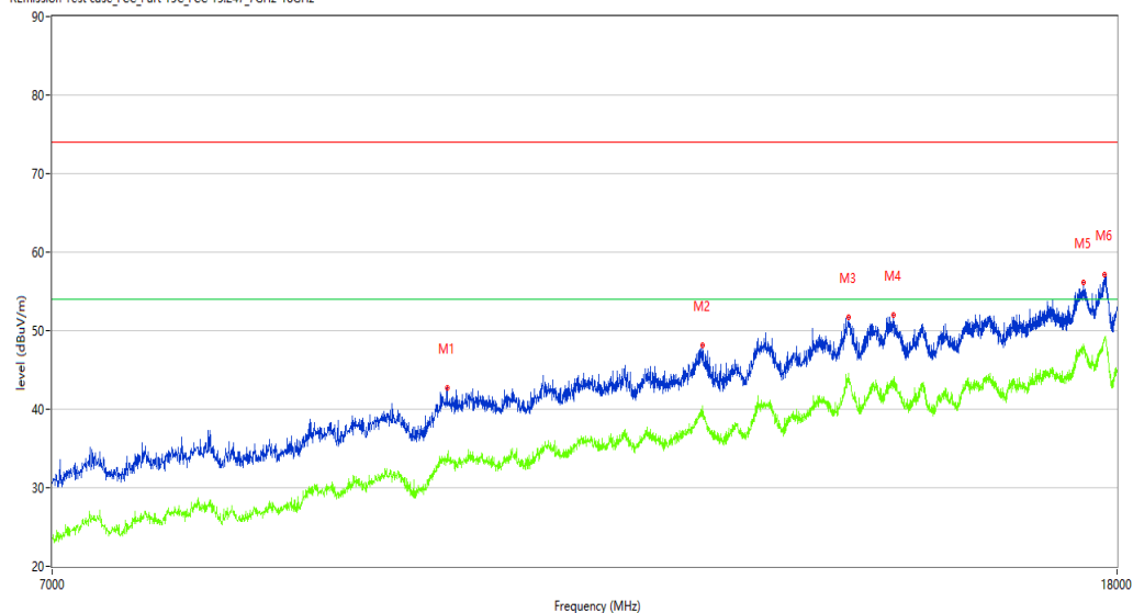
REmission Test case_FCC_Part 15C_FCC 15.247.7GHz-18GHz
