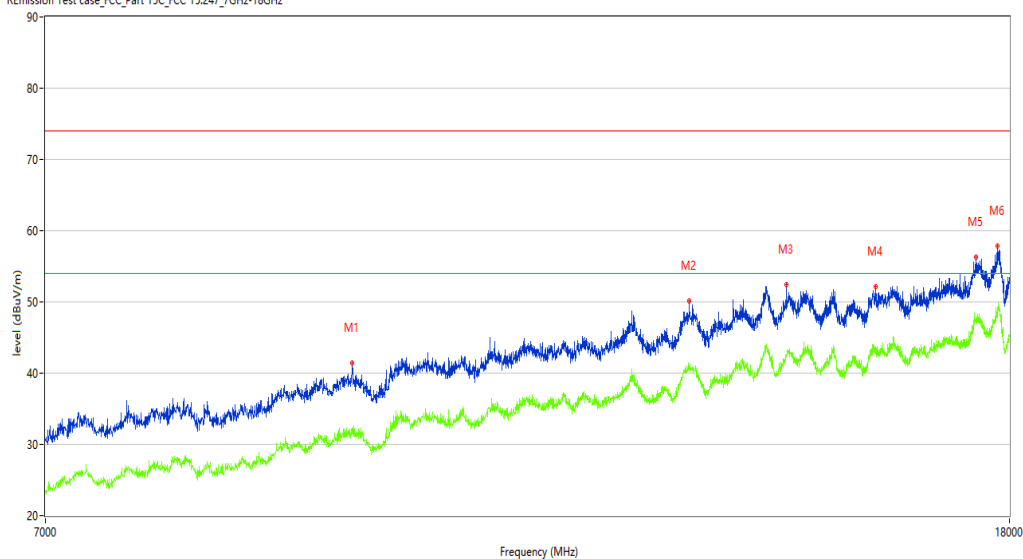
R Emission Test case_FCC_Part 15C_FCC 15.247.7GHz-18GHz
