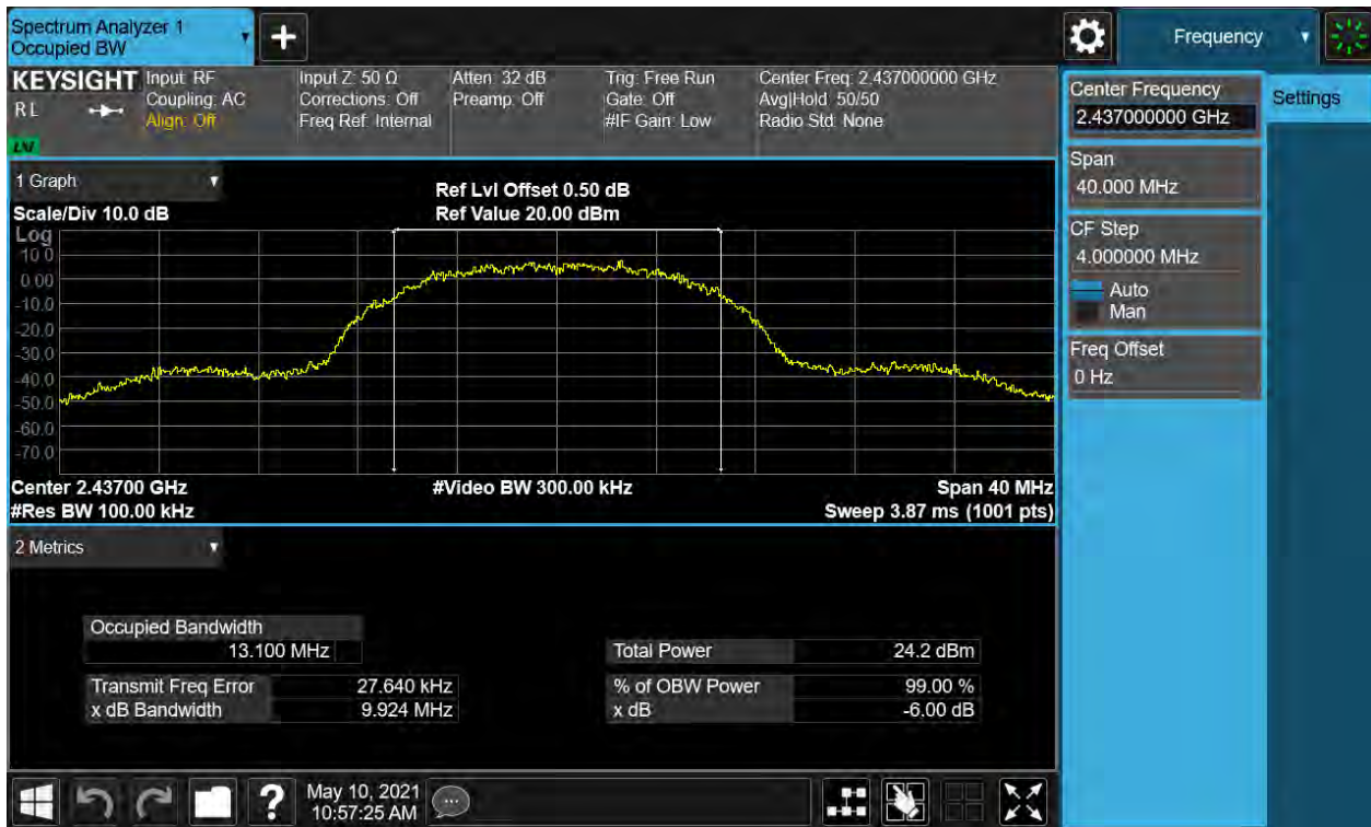
Figure 2: 6dB Bandwidth and 99% Bandwidth, 802.11b, 2437MHz
