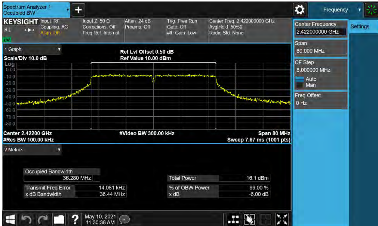
Figure 10: 6dB Bandwidth and 99% Bandwidth, 802.11n(HT40), 2422MHz
