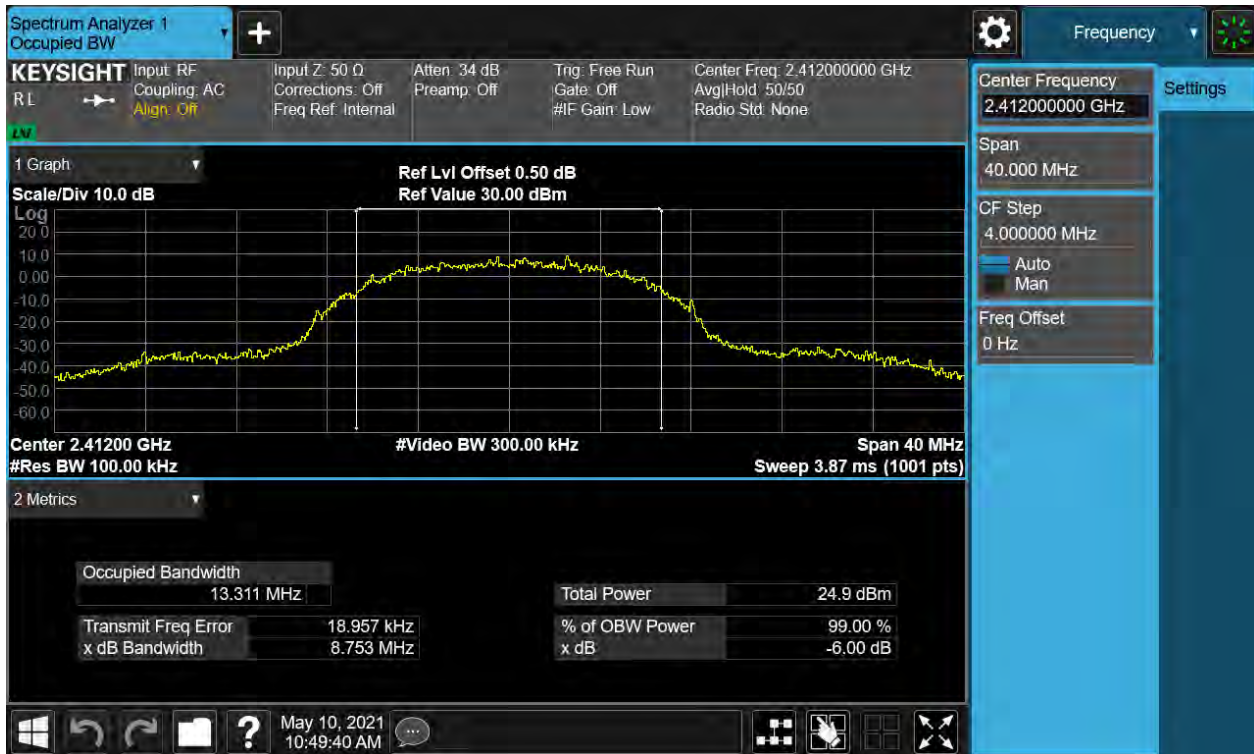
Figure 1: 6dB Bandwidth and 99% Bandwidth, 802.11b, 2412MHz
