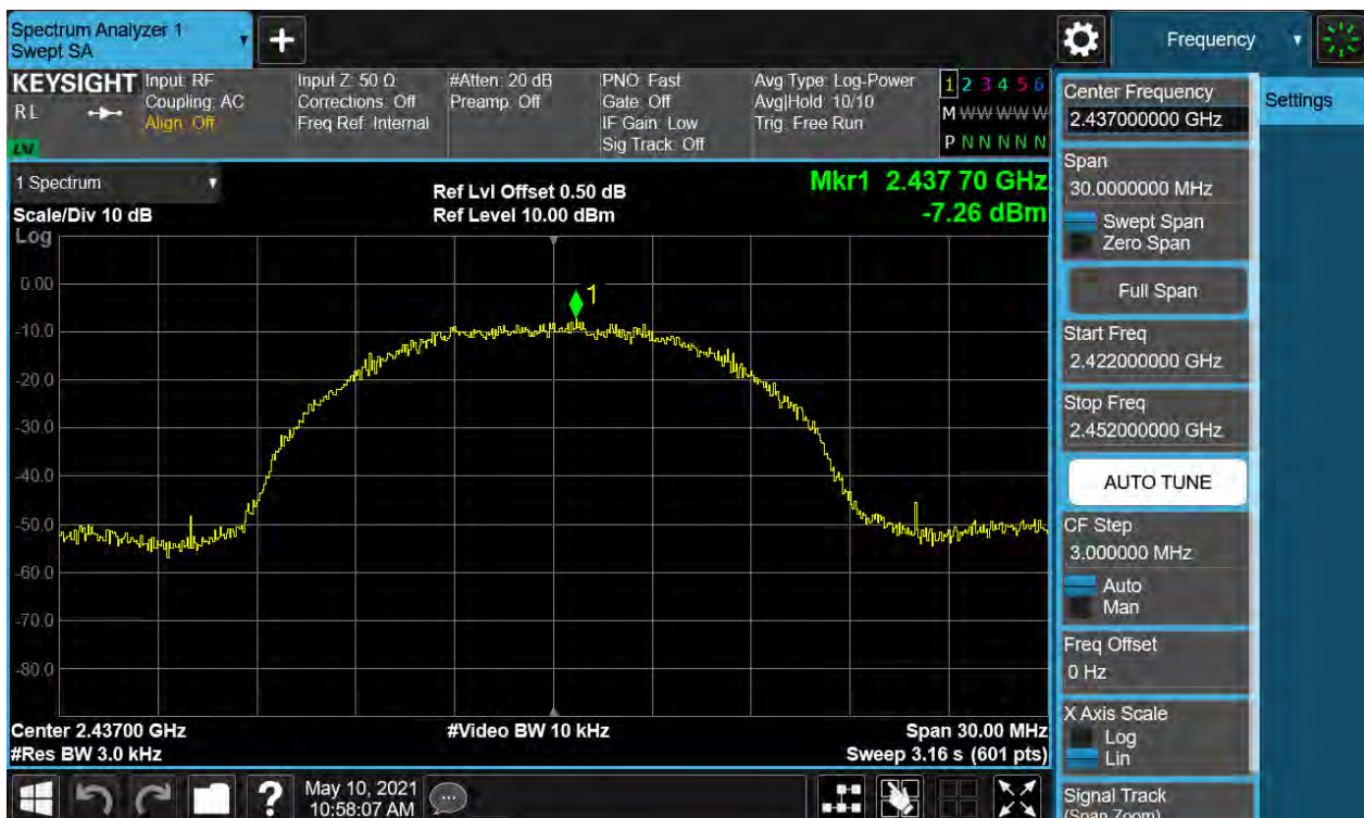
Figure 14: Power Spectral Density, 802.11b, 2437MHz
