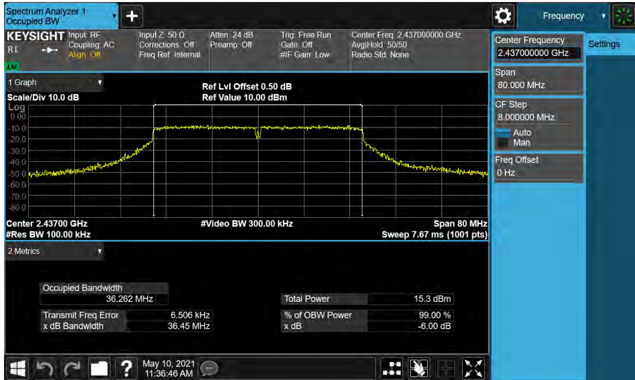
Figure 11: 6dB Bandwidth and 99% Bandwidth, 802.11n(HT40), 2437MHz
