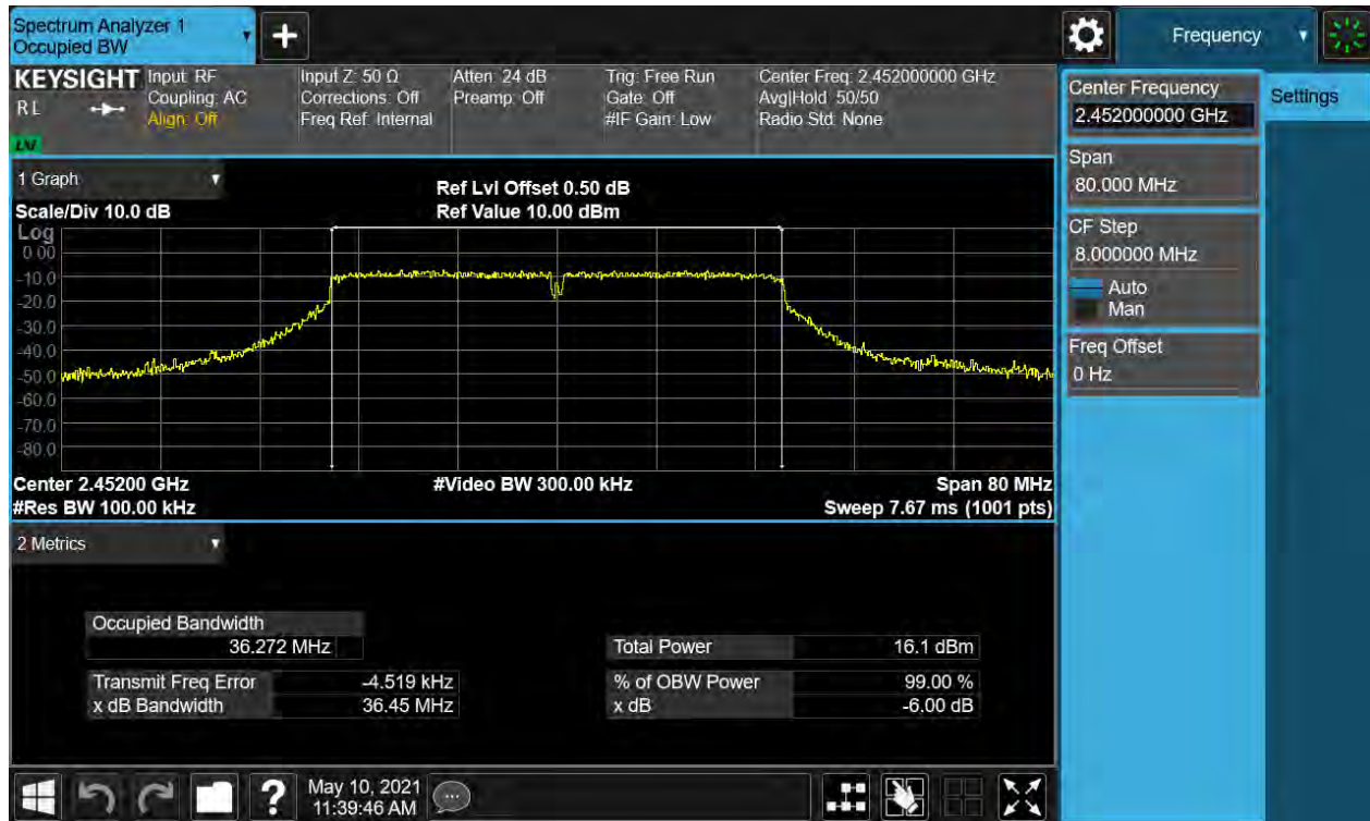
Figure 12: 6dB Bandwidth and 99% Bandwidth, 802.11n(HT40), 2452MHz
