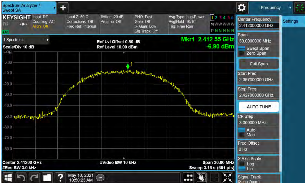
Figure 14: Power Spectral Density, 802.11b, 2437MHz
