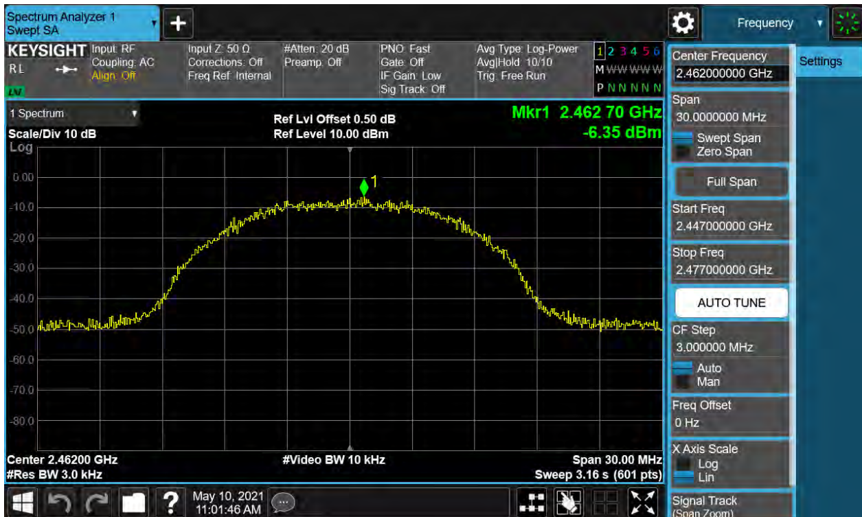
Figure 16: Power Spectral Density, 802.11g, 2412MHz
