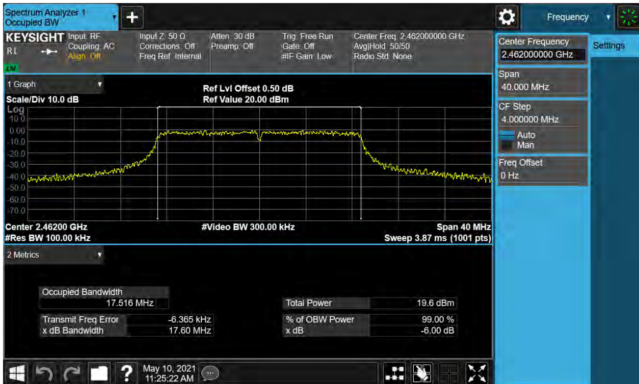
Figure 9: 6dB Bandwidth and 99% Bandwidth, 802.11n(HT20), 2462MHz
