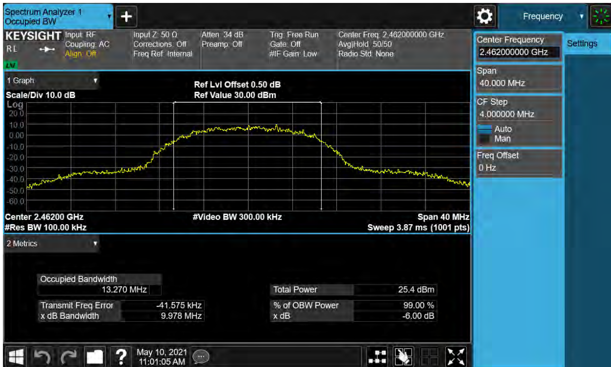
Figure 3: 6dB Bandwidth and 99% Bandwidth, 802.11b, 2462MHz
