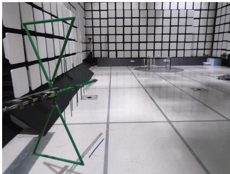
Photograph 4. Radiated Emissions, 30MHz – 1 GHz, Test Setup, Antenna View
