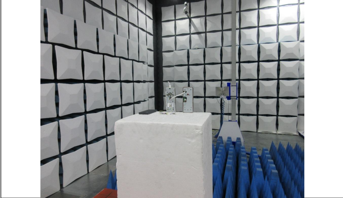
CONDUCTED EMISSION MEASUREMENT SETUP (Below 30MHz)
