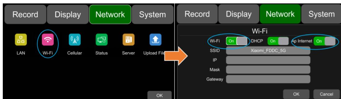
(2) Search and connect to the MDVR Wi-Fi hotspot: The SSID name of MDVR hotspot is prefixed with "WFD-", followed by the serial number of the device (the password is: ap12345678), as shown below:
