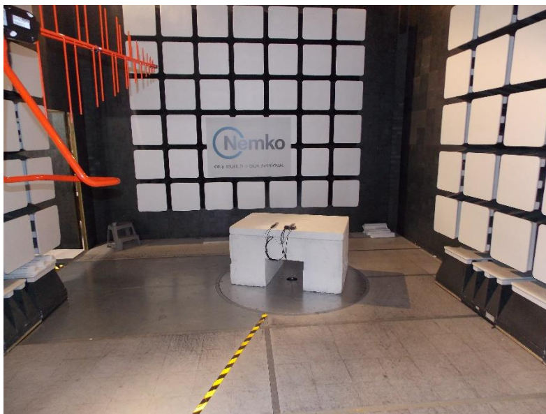
Figure 8.1-3: Radiated emissions setup photo – below 1 GHz
