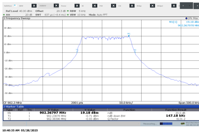
Figure 7.4-1: 20 dB bandwidth on low channel – 125 kHz BW
