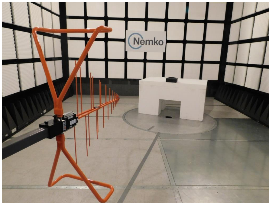
Figure 8.1-3: Radiated emissions setup photo
