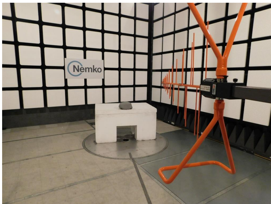
Figure 8.1-3: Radiated emissions setup photo – below 1 GHz
