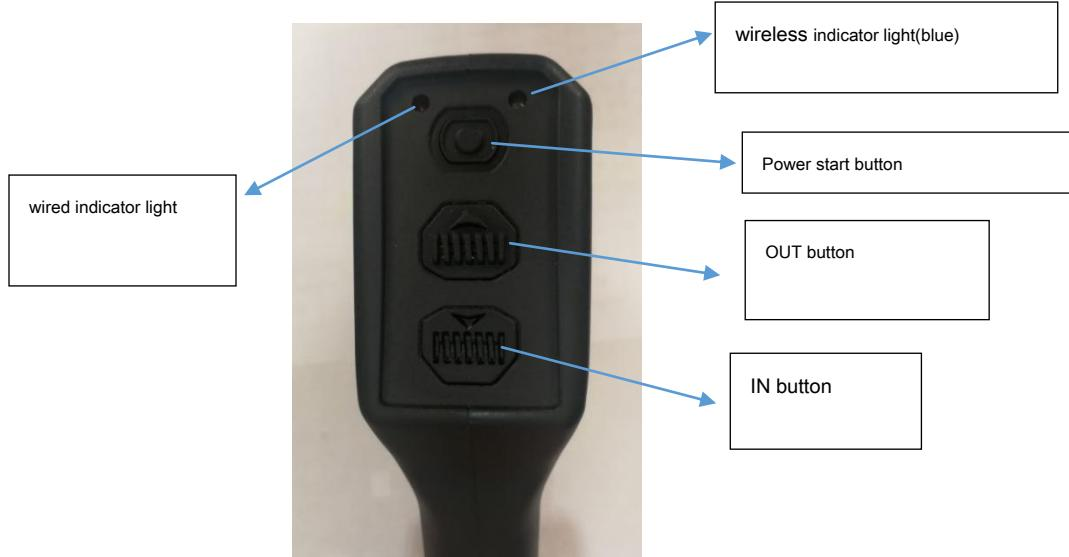
2. Function description: long press the power start button to start for 3 seconds, and the blue wireless indicator lights up. Power off automatically for 2 minutes without any operation. Press the OUT button the blue light flashes winch outgoing (nylon rope/wire rope). Press IN button blue light winch incoming (nylon rope/wire rope). When using wired control, the wireless remote control blue light off, red wired control light on.
