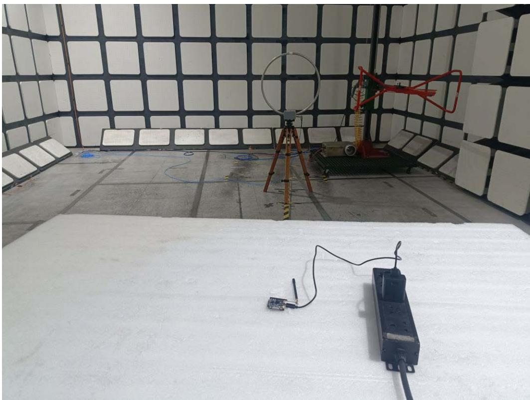
**Radiated Emissions View (30 MHz- 1 GHz) (Antenna1)**
