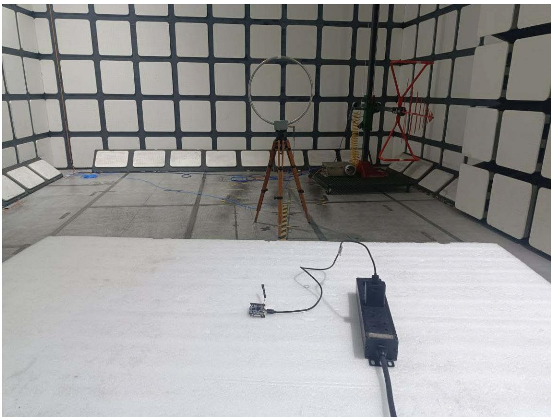
**Radiated Emissions View (30 MHz- 1 GHz) (Antenna2)**
