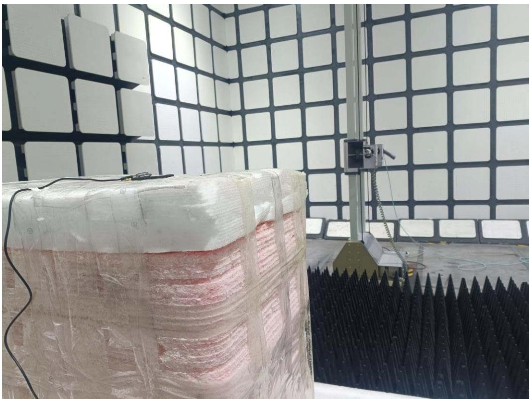
**Radiated Emissions View (9 kHz- 30MHz) (Antenna2)**
