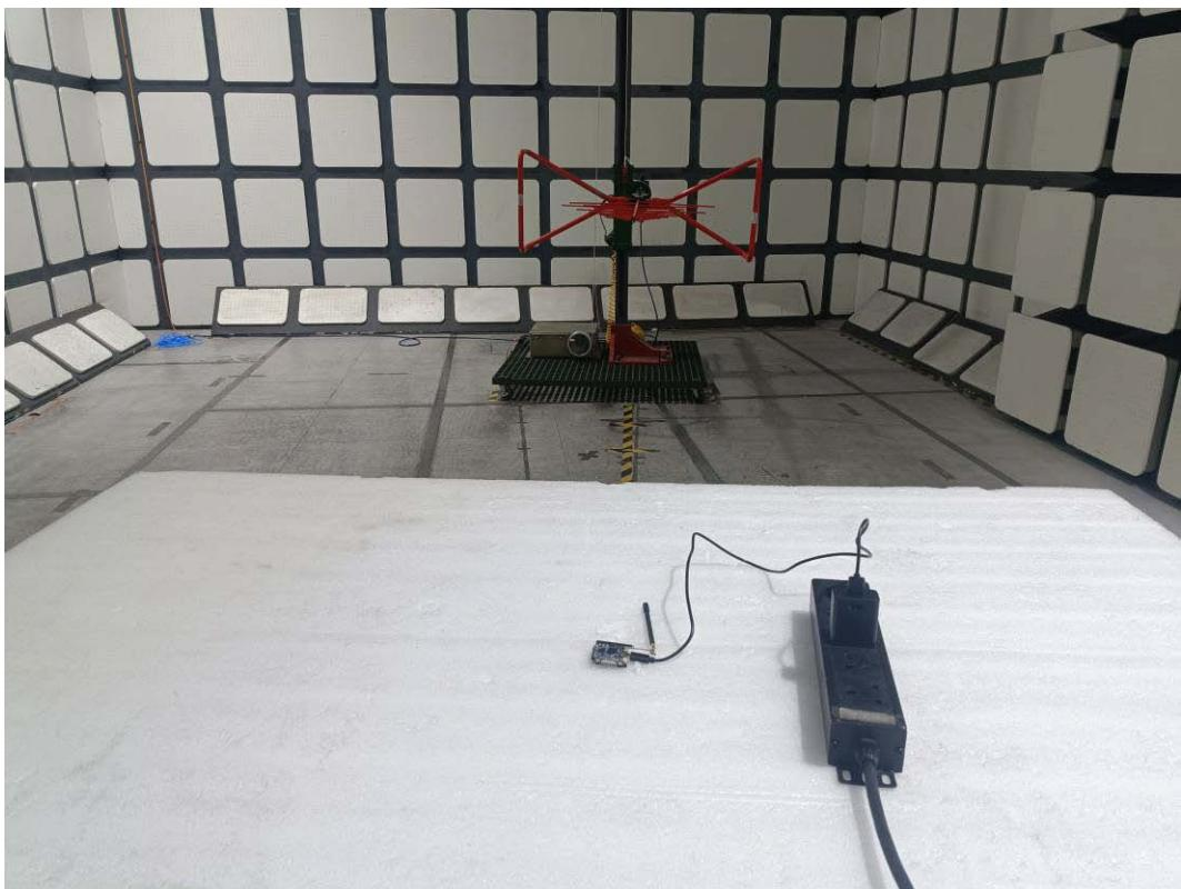
**Radiated Emissions View (Above 1 GHz) (Antenna1)**
