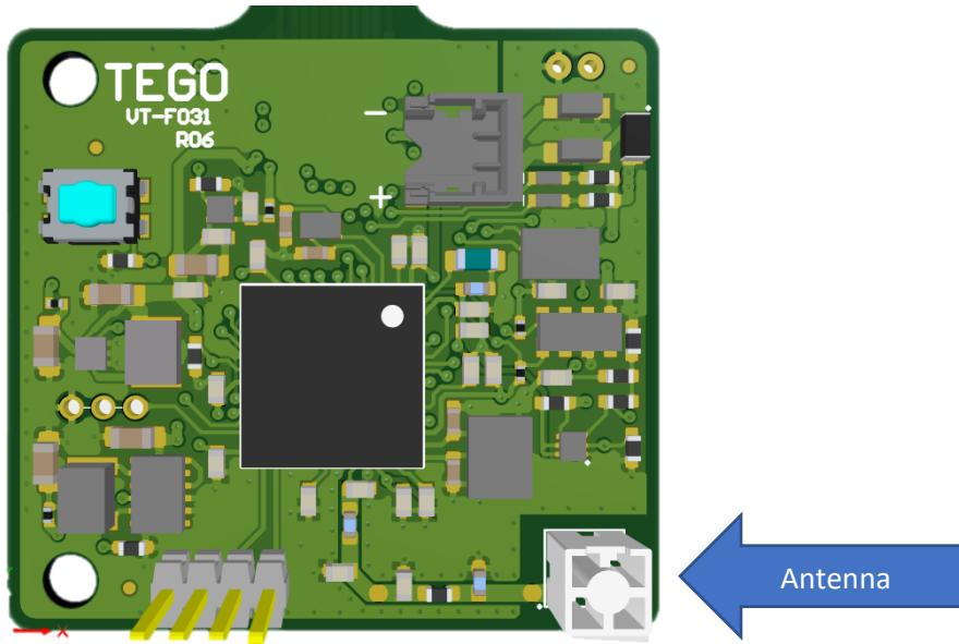
The antenna is a 2.4 GH SMD On-Ground Antenna, with an absolute peak gain of 3.7dBi.
