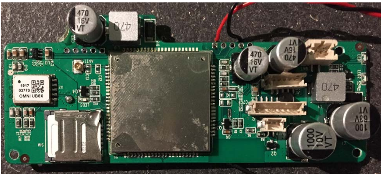
Main Board Top View Cellular and Wifi certified modules occupy this side.
