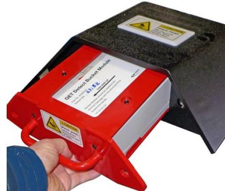
4. Secure the Bucket Module Cartridge Assembly to the Bucket Shield using the two (2) M14 socket head cap screws and a 12mm hex bit.
