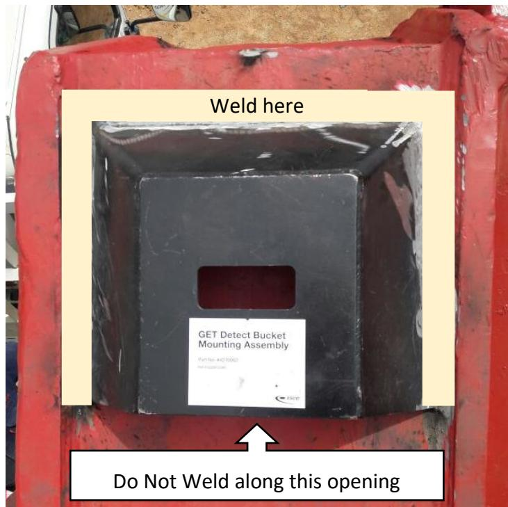
6. After the weld has cooled, paint or otherwise protect the weld area in accordance with the work site's recommended practice (optional).
