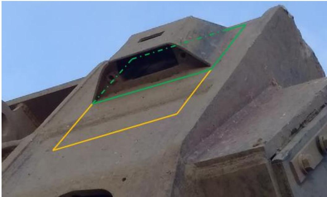
5. Position the Bucket Shield such that any gussets or ribs on the bucket structure do not impede access to or removal of the Bucket Cartridge.
