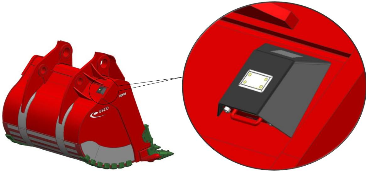
3. The Bucket Shield should be visible to the operator at some time during normal machine use, preferably during the bucket dump cycle.
