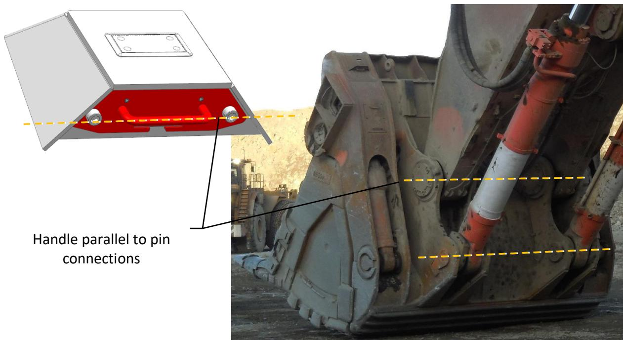
2. Locate the Bucket Shield near the top of the bucket, out of the material flow path, and to the far right or left side. Example locations for both face shovels and hoe excavators are shown below:
