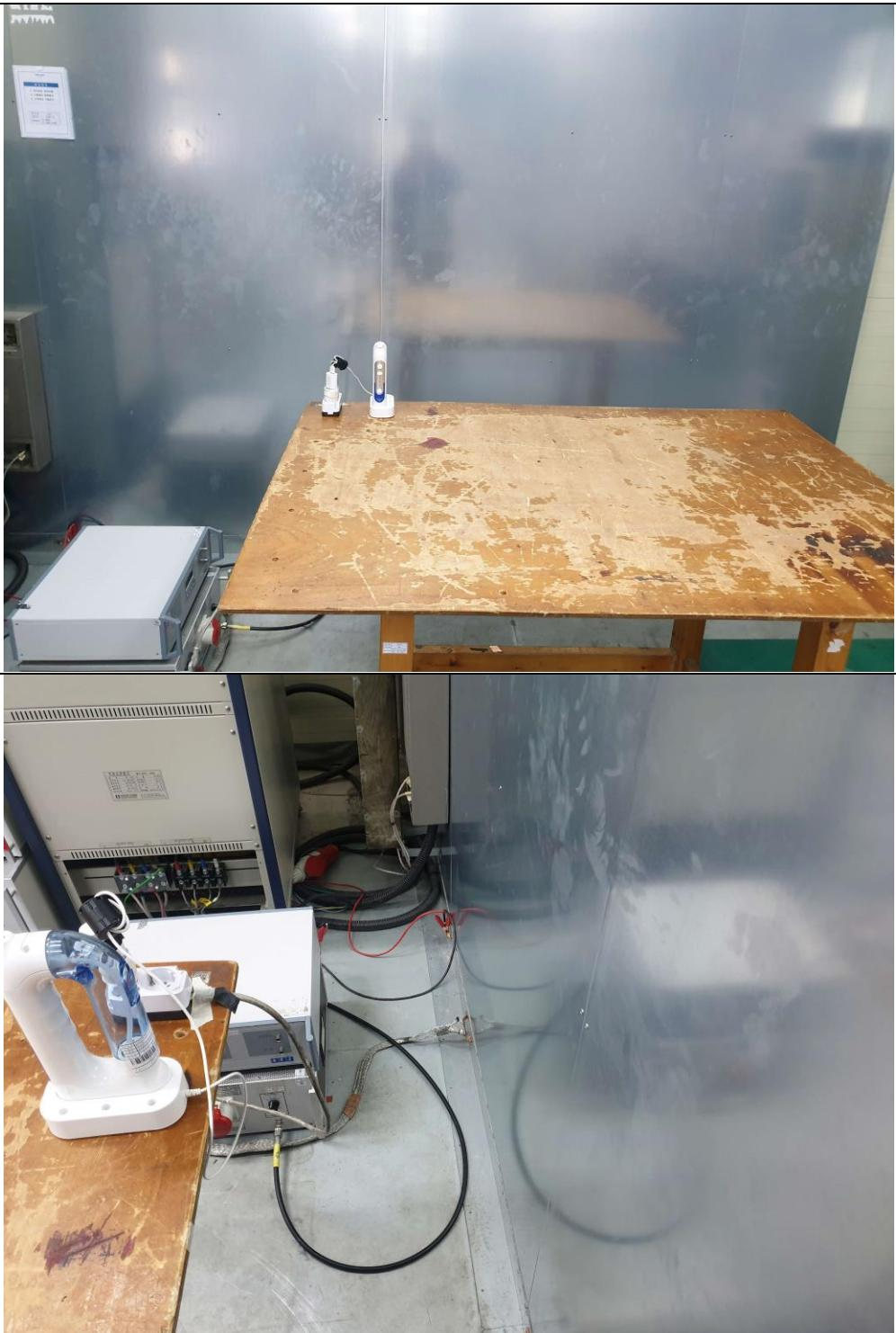
**Radiated Emission Test Set Up (Below 1 GHz)**
