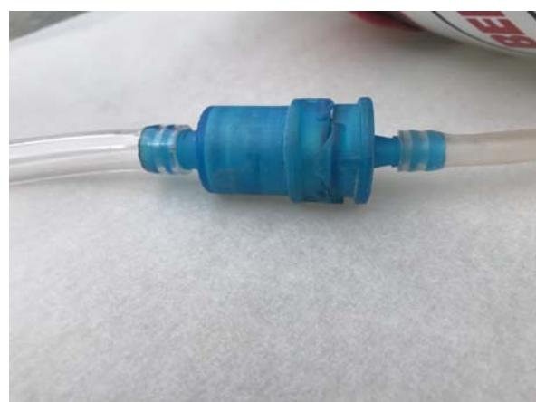
7. Pull the helmet tube from the nozzle and suck on it to raise water through the pump and through the backflow connector. This keeps the pump primed and eliminates air from the pump. The pump is not self-priming. Always make sure water is in the tube above the pump before using.
