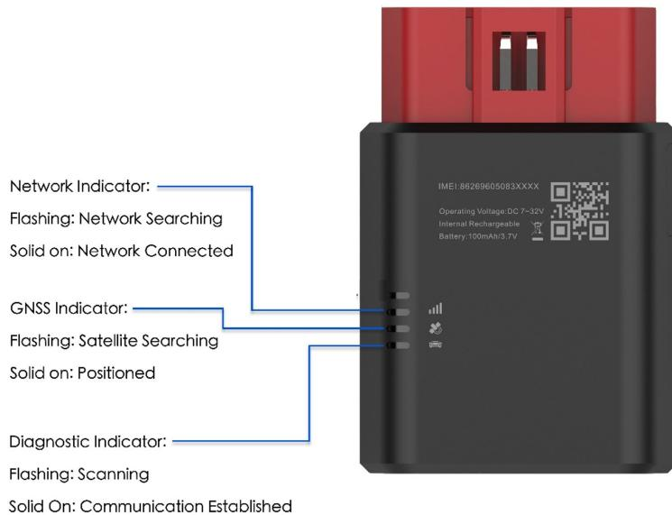
Note: Indicator lights will go out automatically after the tracker turns on for 8 minutes.
