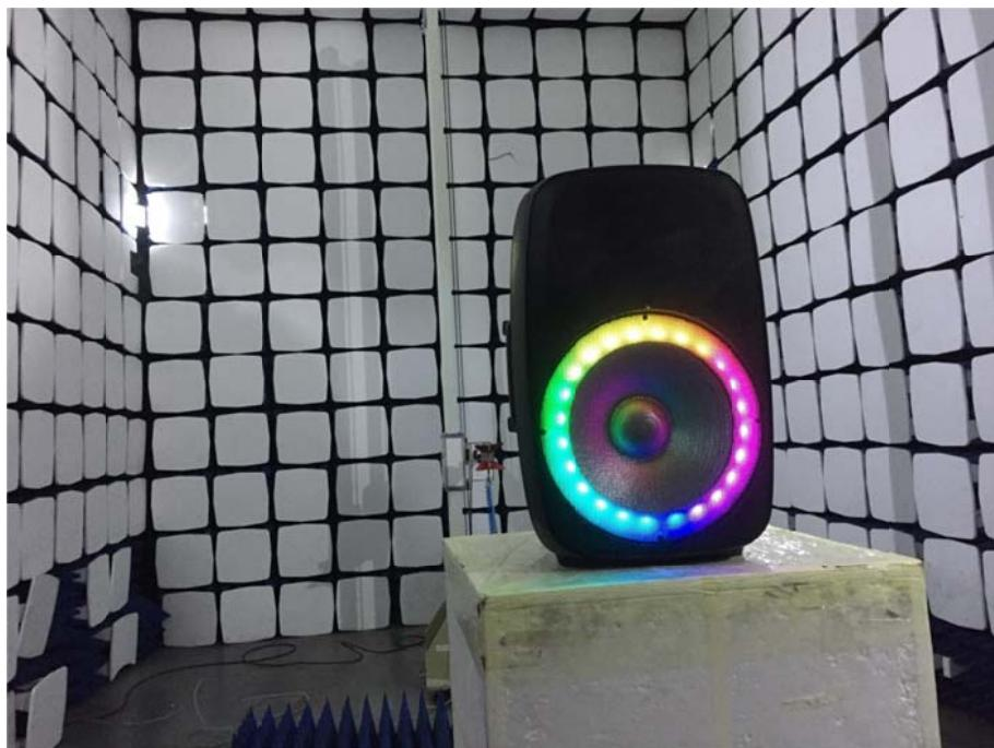
**Radiation Emission Test Setup (Above 18GHz)**
