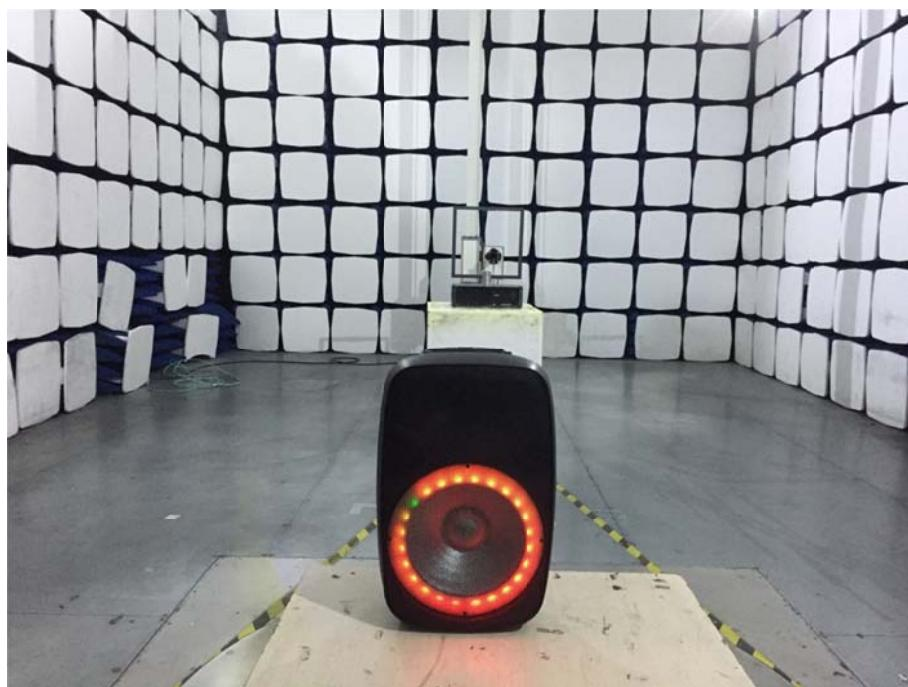
**Radiation Emission Test Setup (30MHz to 1GHz)**
