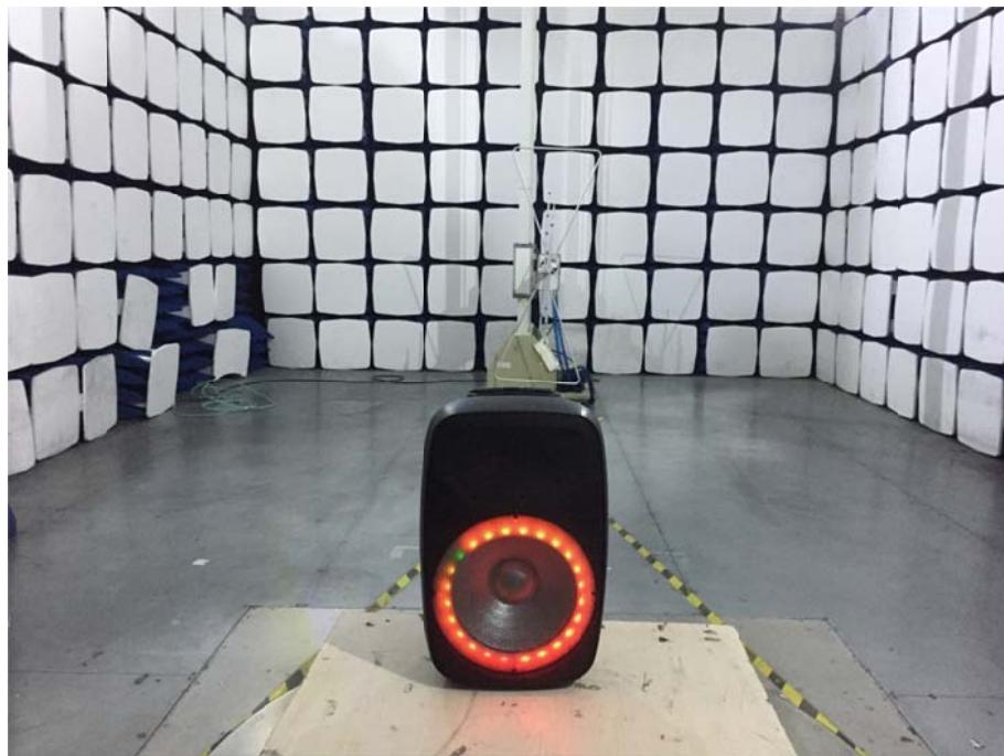
**Radiation Emission Test Setup (1GHz to 18GHz)**
