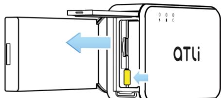
**2** Press the yellow latch so that the battery can be released. Pull the battery tab to slide out the battery.
