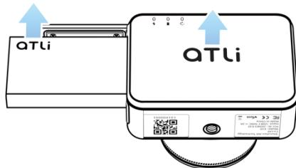
**3** Use the battery to push the yellow latch back until the battery can be inserted.
