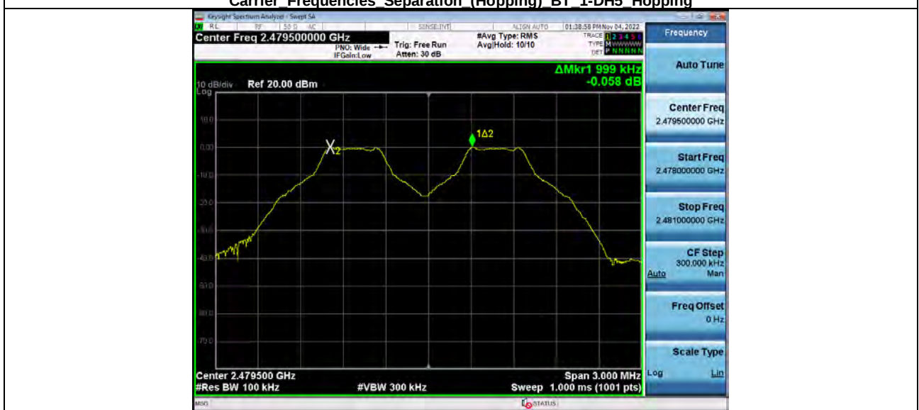
Carrier Frequencies Separation (Hopping) BT 2-DH5 Hopping
