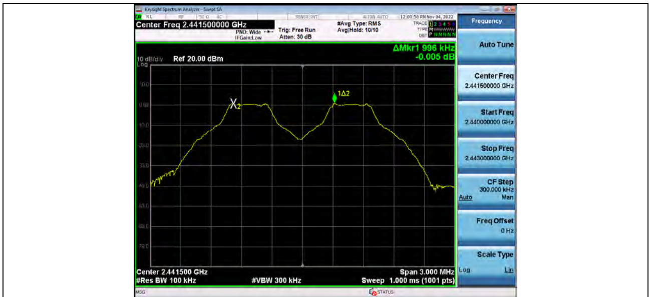
Carrier Frequencies Separation (Hopping) BT 1-DH5 Hopping
