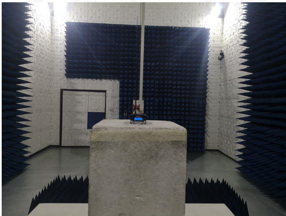
RADIATED EMISSION TEST SETUP –BELOW 1GHz
