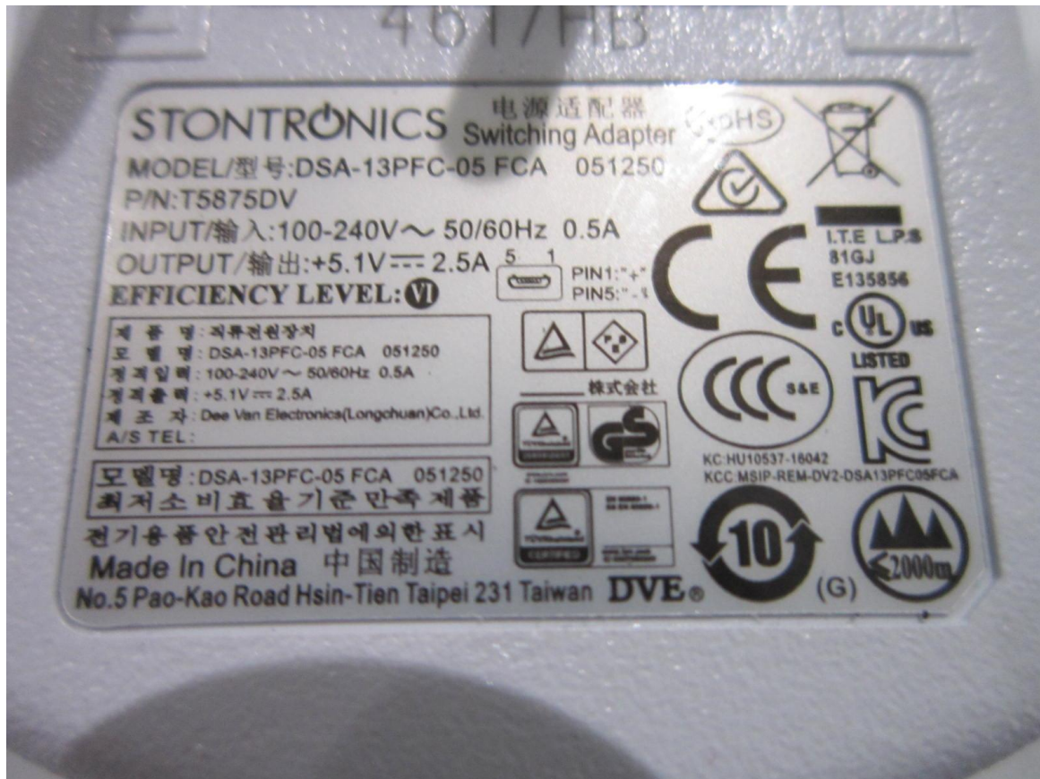
External AC/DC power adapter label Model DSA-13PFC-05 FCA (not included)
