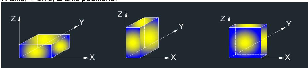
Note: For all radiated test, EUT in one orthogonal axis (X axis) emissions had been tested and recorded in the report.
