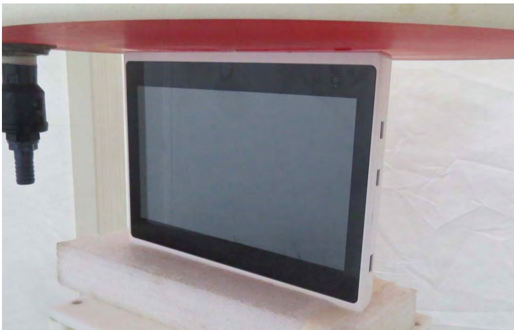
Picture 7: Top Side, the distance from handset to the bottom of the Phantom is 0mm
