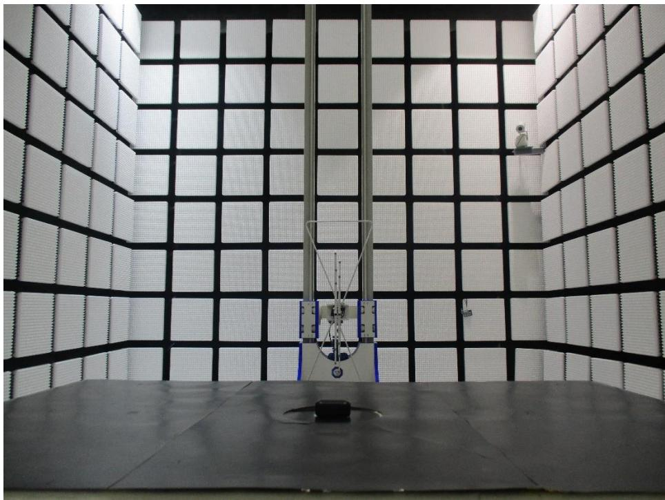
Radiated spurious emission for 30MHz above 1GHz:
