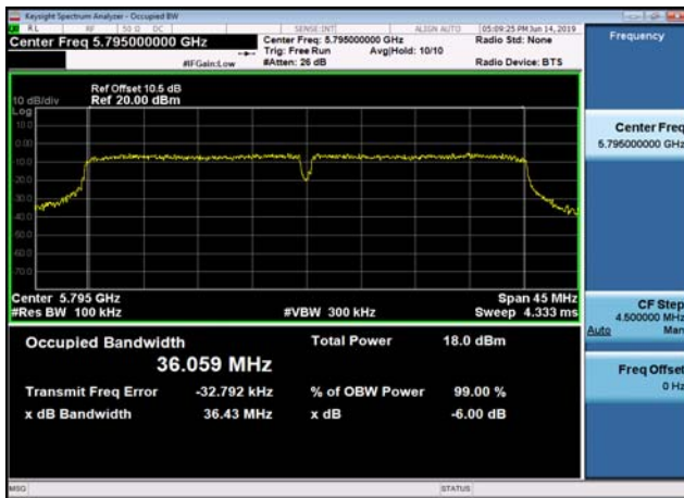
U-NII-3 6dB Bandwidth-802.11a(20MHz) ,5745MHz,Ant0
