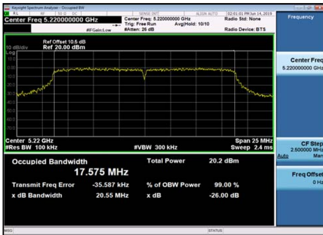
U-NII-1 26dB Bandwidth-802.11ac(20MHz ,5240MHz,Ant0
