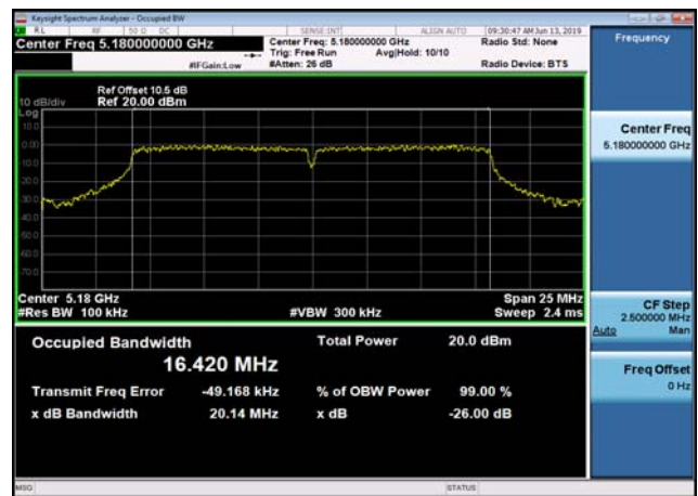
U-NII-1 26dB Bandwidth-802.11a(20MHz) ,5180MHz,Ant1
