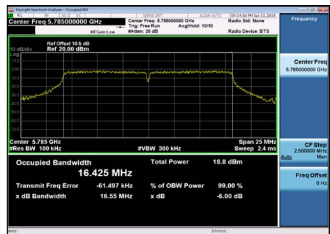
U-NII-3 6dB Bandwidth-802.11a(20MHz) ,5785MHz,Ant1
