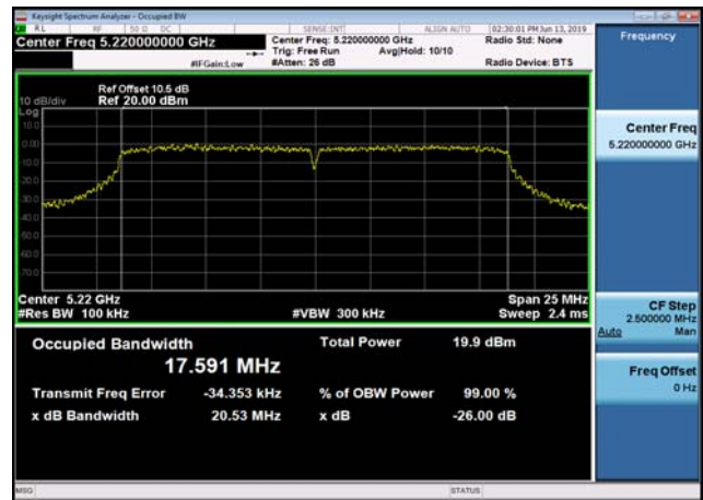
U-NII-1 26dB Bandwidth-802.11ac(20MHz ,5240MHz,Ant1
