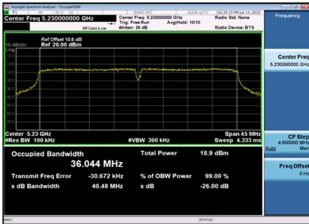
U-NII-1 26dB Bandwidth-802.11a(20MHz) ,5180MHz,Ant0
