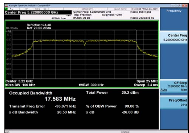
U-NII-1 26dB Bandwidth-802.11n(20MHz) ,5240MHz,Ant1
