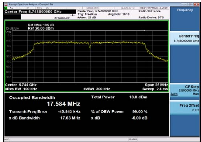
U-NII-3 6dB Bandwidth-802.11ac(20MHz) ,5785MHz,Ant1
