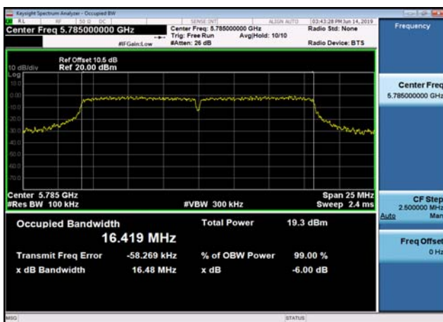
U-NII-3 6dB Bandwidth-802.11a(20MHz) ,5785MHz,Ant0
