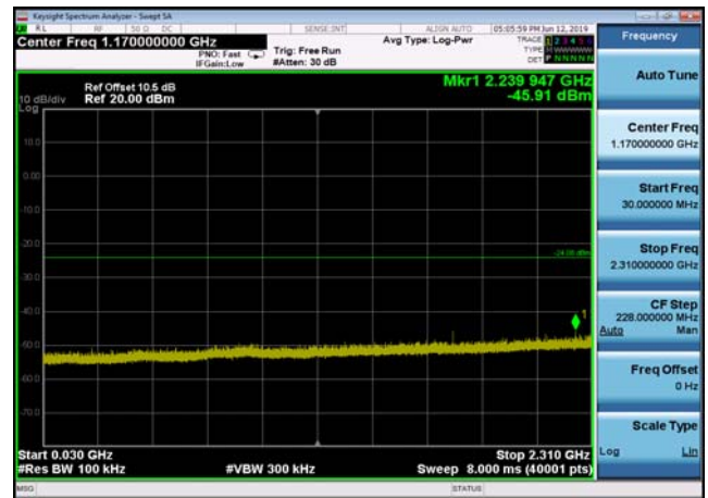
,Plot 3,30MHz~2310MHz-802.11g,2437MHz ,Ant1
