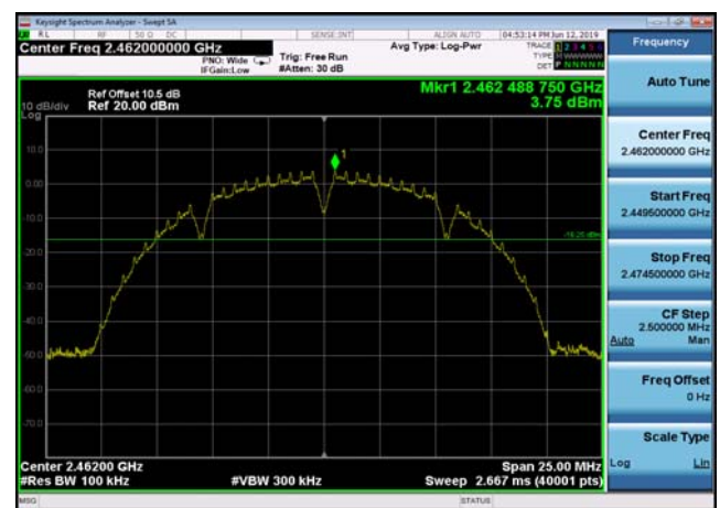
,Plot 1,Reference Level-802.11b ,2462MHz,Ant1
