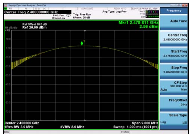
Output Power: DQPSK,2480MHz,2DH5
