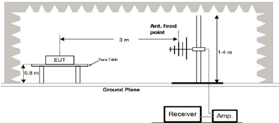
(3) Radiated Emission Test-Up Frequency Above 1GHz
