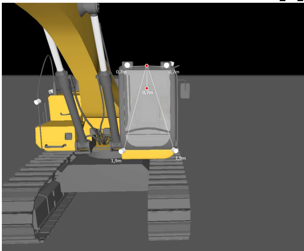
Figure 1 shows typical installation of the system and distances to cockpit
