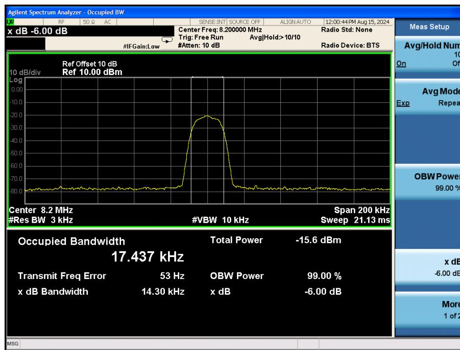
Note: The operating bandwidth of 14.3 kHz at 8.2MHz demonstrates that the fundamental frequency is not overlapping 15.205 restricted bands.
