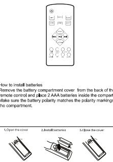
How to install batteries
