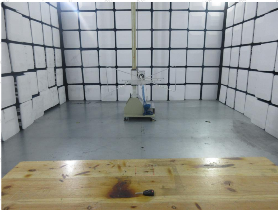
Photo of Radiation Emission Test
