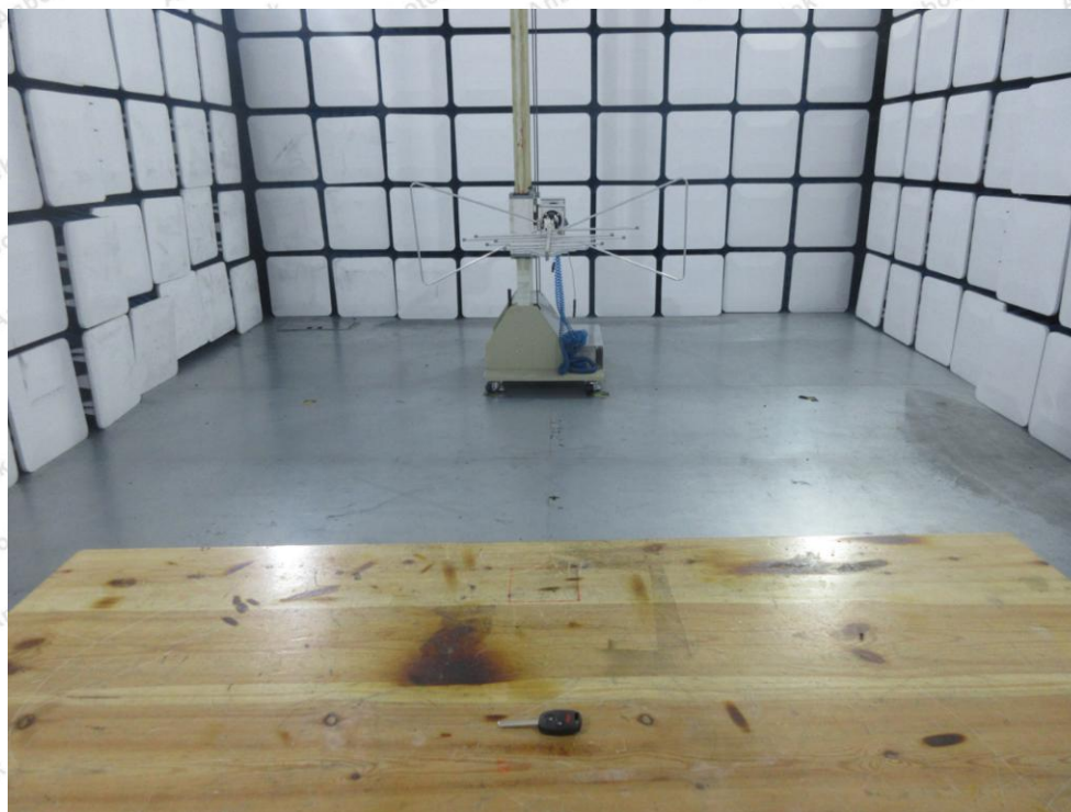
Photo of Radiation Emission Test
