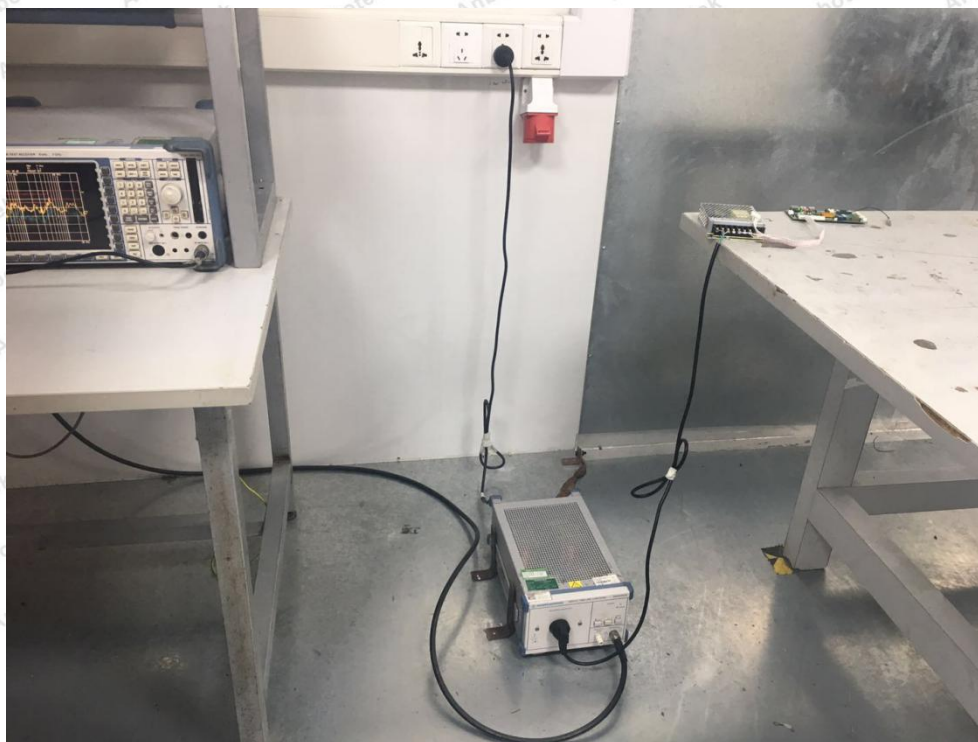
Photo of Conducted Emission Measurement
