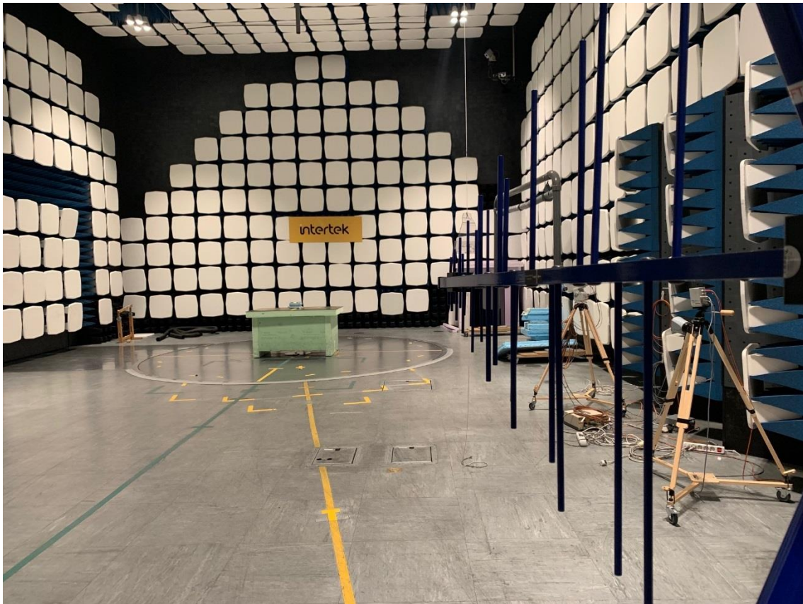
Test set up radiated emission 30 MHz – 1GHz
