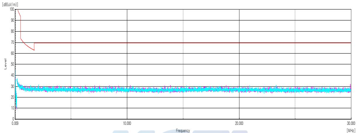
**Test results (Below 1 000 MHz) – Worst case: 802.11a\_UNII-1 Highest frequency**
